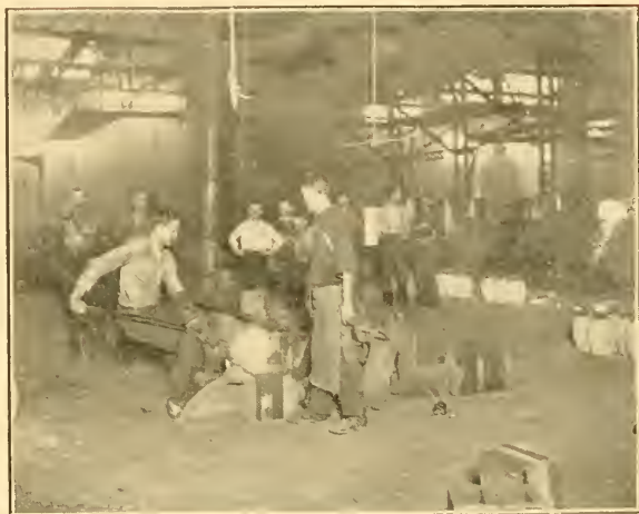
MAKING CRUCIBLE INGOTS FOR SAW STEEL
